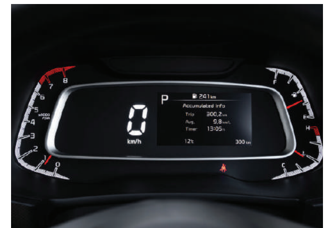
4.2-inch instrument cluster and colour display
